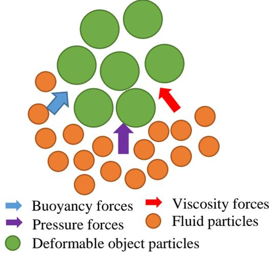
Figure 1. Illustration of the forces for deformable solid particles.
